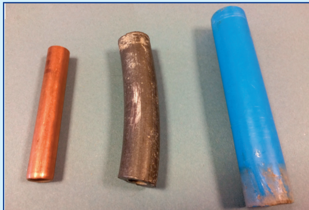
From left to right: copper, lead, hydrodare (plastic) pipes
